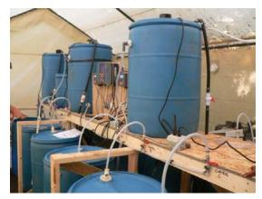
**Figure 2.** Mixing tanks and bio-barrels. Photo by RNT Consulting Inc.
