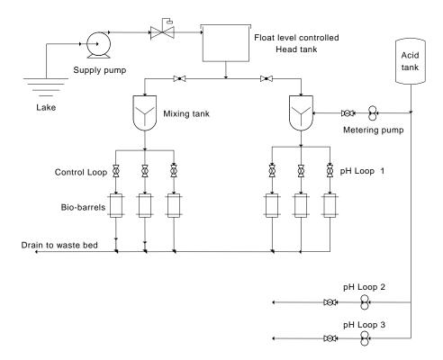
Water exiting each mixing tank was split into three streams. Each stream was directed into a 175 L bio-barrel which contained settlement substrates and mesh bags containing adult mussels. In each bio-barrel, the water entered at the top of the barrel and exited at the bottom. This arrangement resulted in one control and three treatments. Each treatment and the control had three replicates.
