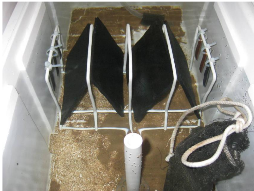
Figure 2. Settlement chamber with settlement plates, corrosion coupons, and mesh bag containing live adult mussels.
