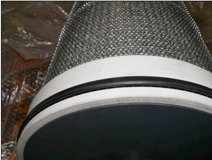
• Figure 8: Seal at backwash end of filter as received
