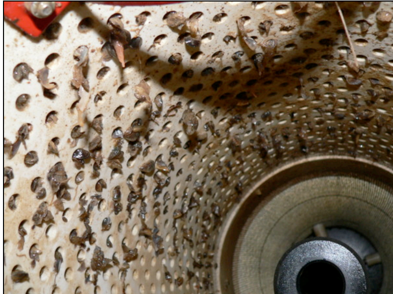
• Figure 10: Inside of pre-strainer showing damaged mussels from Hayward strainer entering Ballast Safe filter.
