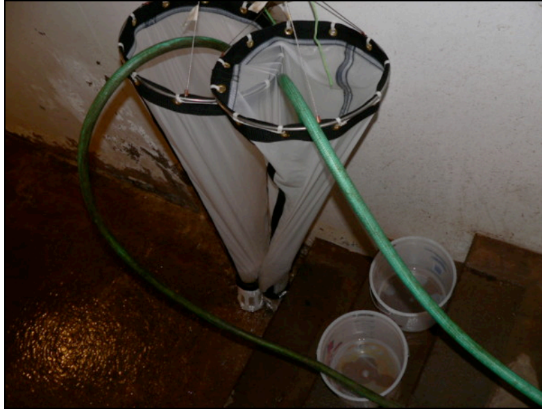
• Figure 5 : Test sample 20 micron collection nets
