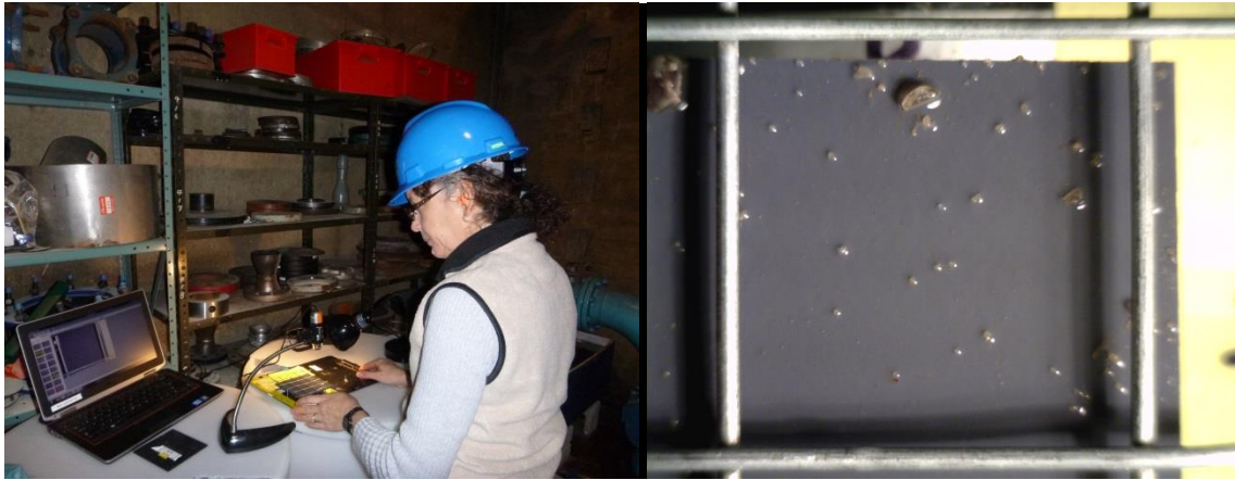
Figure 5. An MBI field scientist (at left) uses the digital microscope method to collect photos of settlement plates (example at right).
